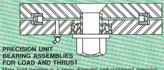
Main load bearing is a large diameter self-contained precision roller bearing. Secondary load bearing is a tapered roller bearing. Both bearings are replaceable as complete assemblies. Recommended for continuous, extra duty service.
