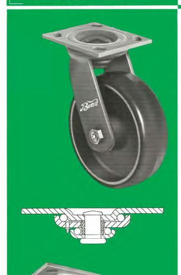
The Series 48-A offers the same top plate size and bolt hole spacings as the Series 46-A except that heavier steel sections are used. This double ball race caster is recommended for use on a wide variety of portable equipment. They are also excellent for warehouse trucks and dollies, portable racks and shelving, as well as for light duty towline trucks.
