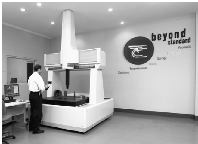
A 1200 x 1000 x 800mm Sheffield Coordinate Measuring Machine is used to inspect parts and assemblies for precision fit.
