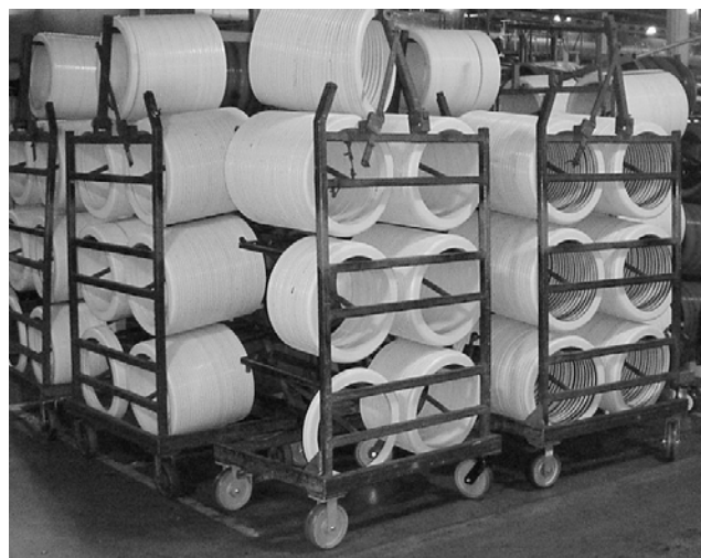
Cantilever racks holding parts for production with 51 Series casters.
